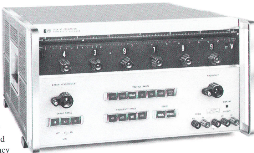
Fig. 2. This new Model 745A AC Calibrator is a precision signal generator designed to provide ac voltages to \pm 0.02\% accuracy at midband. Frequency range is continuously adjustable from 10 Hz to 110 kHz. The percent error scale enables direct error measurement without the necessity for calculation. Voltage, frequency, error ranges and frequency vernier may be programmed.
